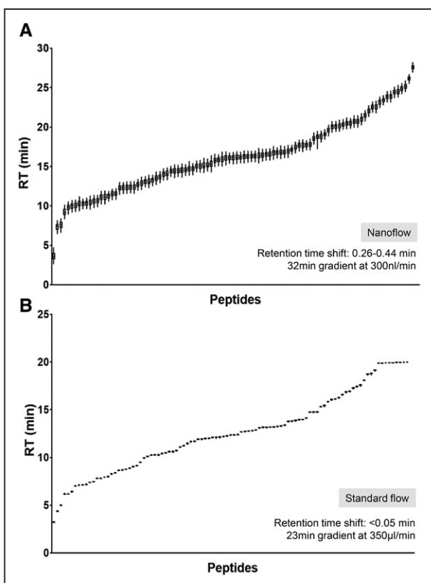
**Figure 4.** Comparison of retention time (RT) between nanoflow and standard-flow liquid chromatography (LC). The RT of each peptide showed higher variation across 668 samples using nanoflow LC (A) compared with standard-flow LC (B).
