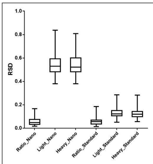
**Figure 3.** Comparison of relative SD (RSD) between nanoflow and standard-flow liquid chromatography (LC). The quality control samples on the nanoflow and standard-flow system showed similar RSD of the light/heavy ratio, but the light or heavy peptide peak area showed a higher variation on the nanoflow system.
